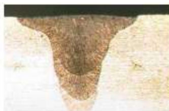
Cross section of penetration; thickness: 2.0 mm (penetrate possible)
